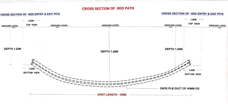
CROSS SECTION OF HORIZONTAL DIRECTIONAL DRILLING
